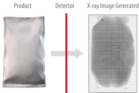
Figure 6: X-ray Image Generation
